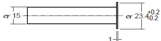
Fig. 9. Pipe (dia 15 mm) for flat sealing ring connection for G 3/4 " external thread
